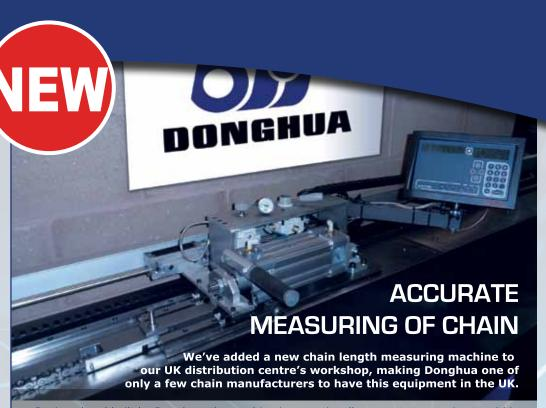
Designed and built by Donghua, the machine is exceptionally accurate measuring to within 10 microns per metre (a human hair is 80-100 microns width) and is capable of measuring up to five metres of chain. The equipment can also pre-load (pre-stretch) chain, eliminating the initial elongation often found in built 'in-house' attachment chain. This means Donghua's attachment chain is ready and easy to fit from the box and with the best possible service life.
